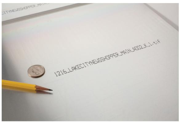
(Easily identify plate signature, color, sequence and direction for punching with the NXP-Tag It printing plate inkjet ID system.)
